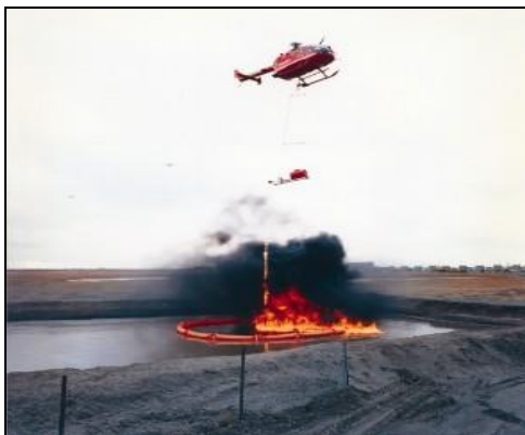
(Helitorch dispensing gelled diesel)
